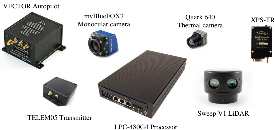
Figure 10.1: Individual units of both the basic and advanced avionics packages.
